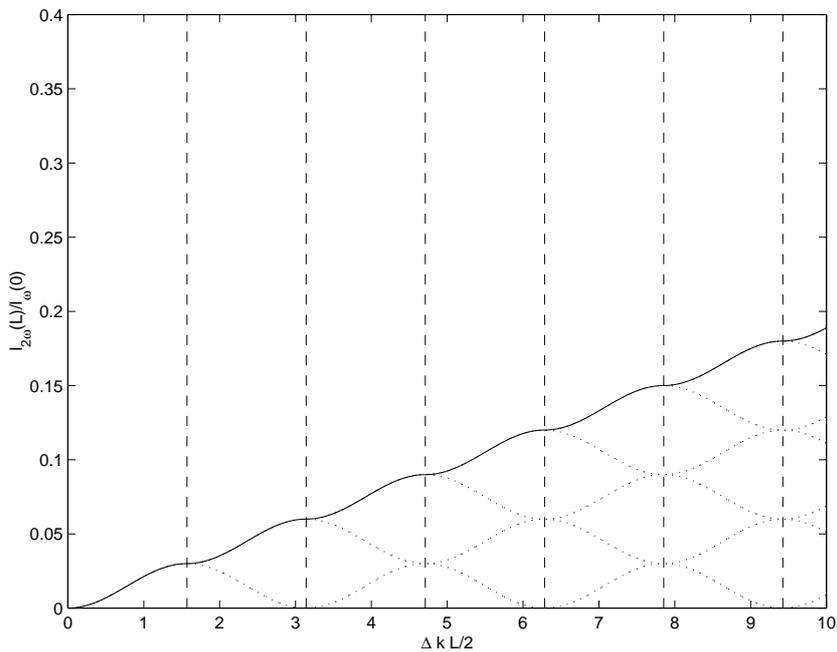
Figure 4. Conversion efficiency  $I_{2\omega}(L)/I_{\omega}(0)$  as function of normalized crystal length  $\Delta k L/2$  when the material properties are periodically reversed, with a half-period of  $L_c$ .
