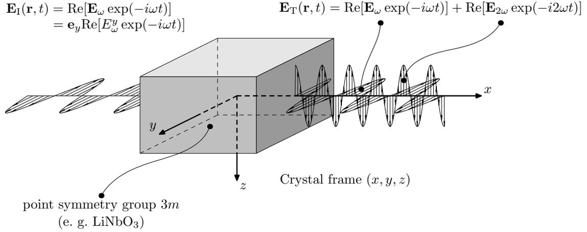
Figure 1. The setup for optical second harmonic generation in LiNbO<sub>3</sub>.
